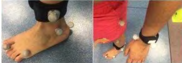
Figure 1. MOCAP and IMU sensors placed in ankle and wrist.
